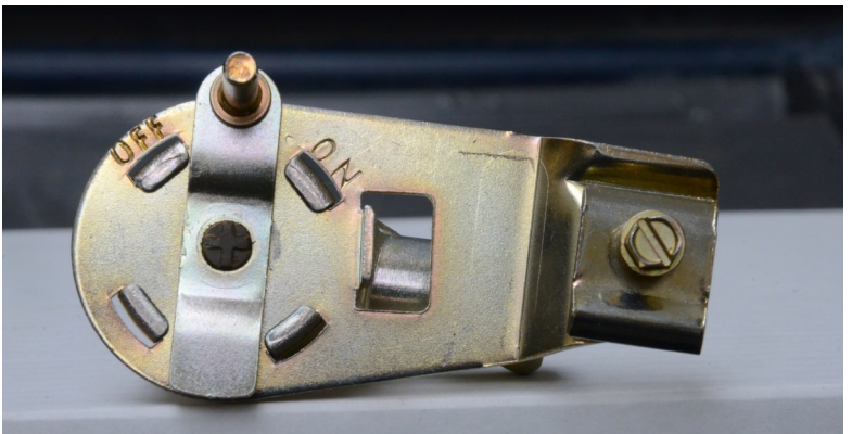
Above and below: Universal replacement heater valve uses ball valve and is similar size and configuration to stock valve.
