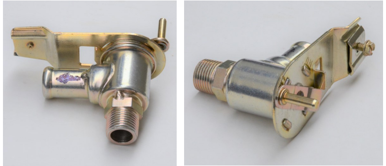
Above and below: Universal replacement heater valve uses ball valve and is similar size and configuration to stock valve.
